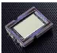
Fujifilm Super CCD Area Type imaging chip
