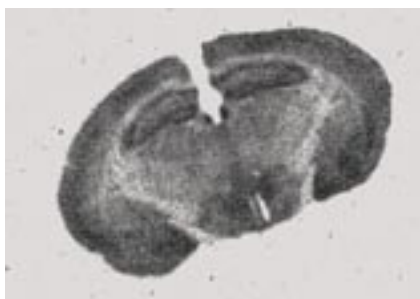
Rat brain autoradiography by BAS-TR plate Sample: 3 H-labeled receptor assay FLA-5100: IP-S mode, Pixel size: 25µm. IP: BAS-TR type
