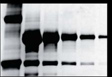
Silver-stained protein by SDS-PAGE Sample: BSA/Density: molecular-weight marker, 3µg, 1µg, 300ng, 100ng, 30ng/Excitation wavelength: 473nm/Filter: Y520/ PMT-1, 500V/Pixel size: 50um
