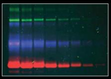
Multiplexed fluorescent protein SDS-PAGE Sample: Green: Cy™3 labeled BSA (laser: 532nm/filter: 0580) Blue: Cy<sup>™</sup>2 labeled Carbonic anhydrase (laser: 473nm/filter: Y520) Red: Cv<sup>™</sup>5 labeled Lysozyme (laser: 635nm/filter: R670)/PMT-1
