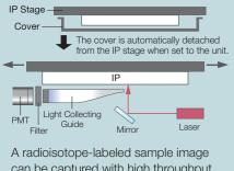
can be captured with high throughput and high sensitivity using Fujifilm's unique proprietary technologies: integrated Imaging Plate technology and high-speed detection technology (Light Collecting Guide).
