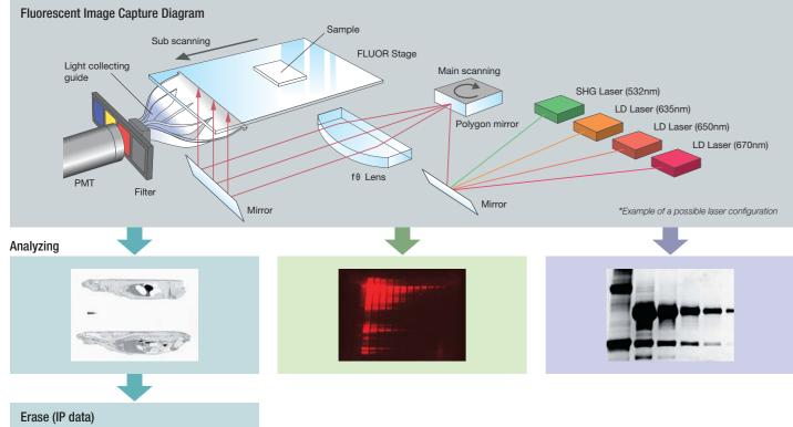
The IP data can be erased and IP is used repeatedly.
